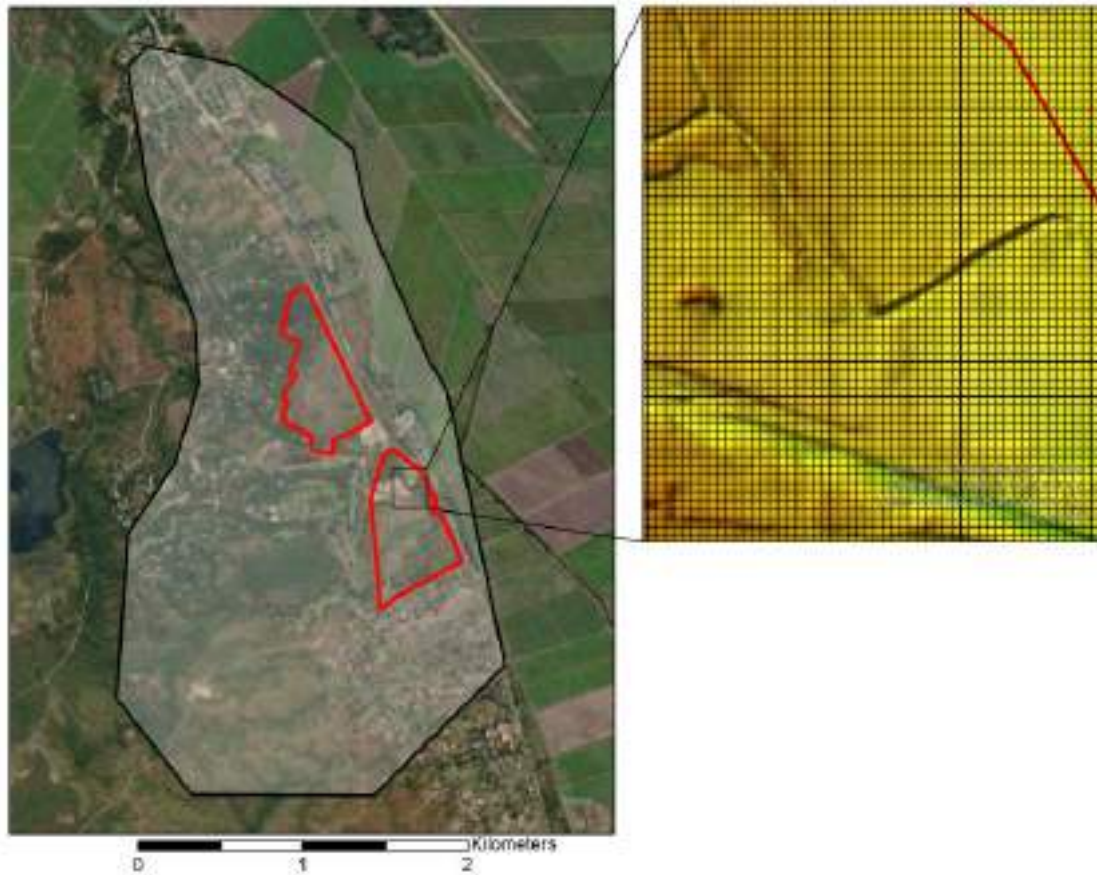
FIGURE 5-8 Extent of modelled area (left), including details of computational grids and underlying terrain used in the hydraulic simulations
