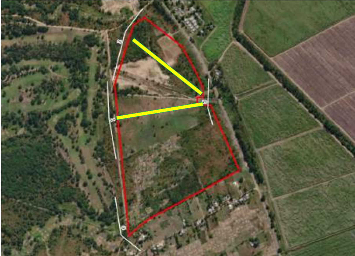
FIGURE 5-13 Culvert alternatives shown with yellow lines
