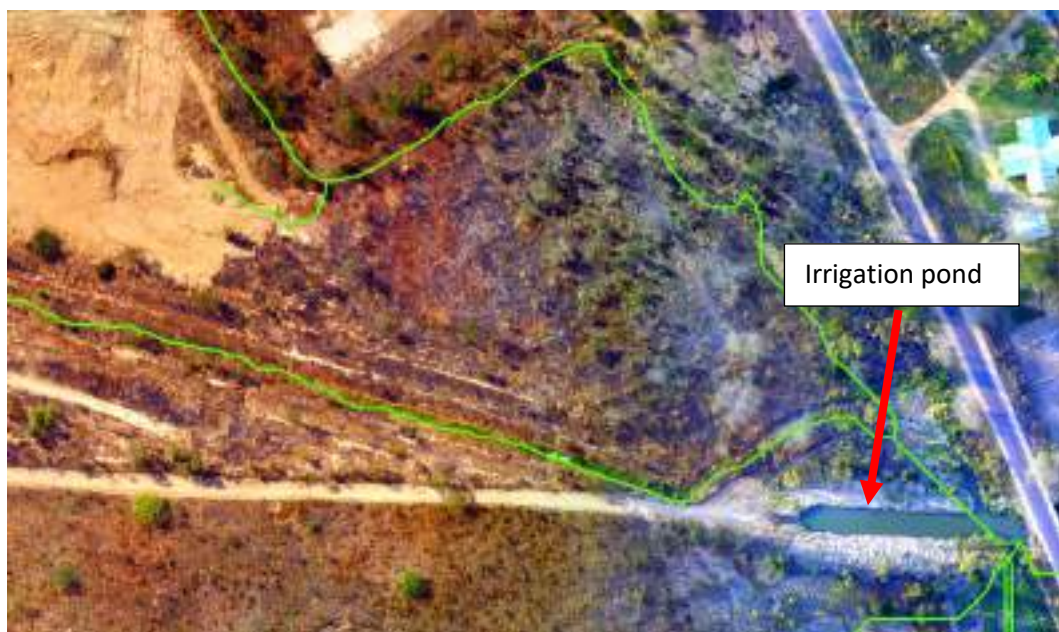
FIGURE 5-5 Drainage lines, shown for parts of the southern plot where the water accumulates towards the irrigation pond. Both the red (3) and white (4) catchment drains towards this area
